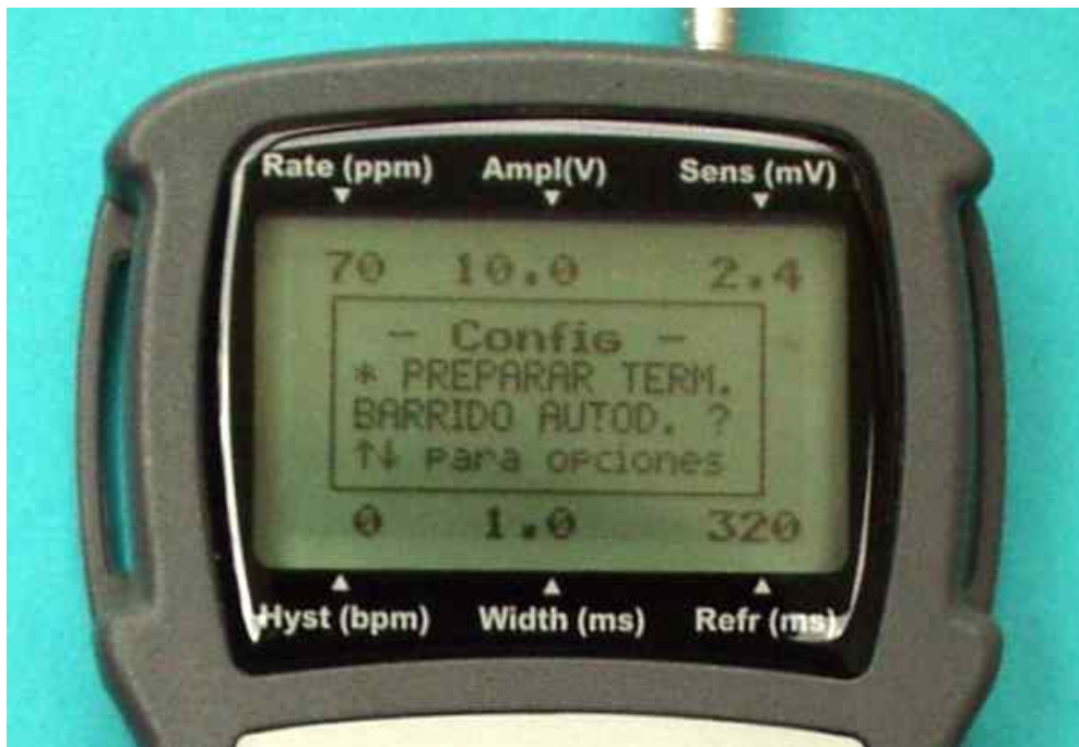
Figure 4.2: Scanning Reversion Parameter Setting (Spanish)
